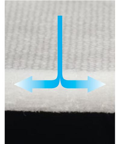
*The fibres in the absorbent layer are arranged horizontally so that they encourage fluid to spread evenly across the full breadth of the pad.*
